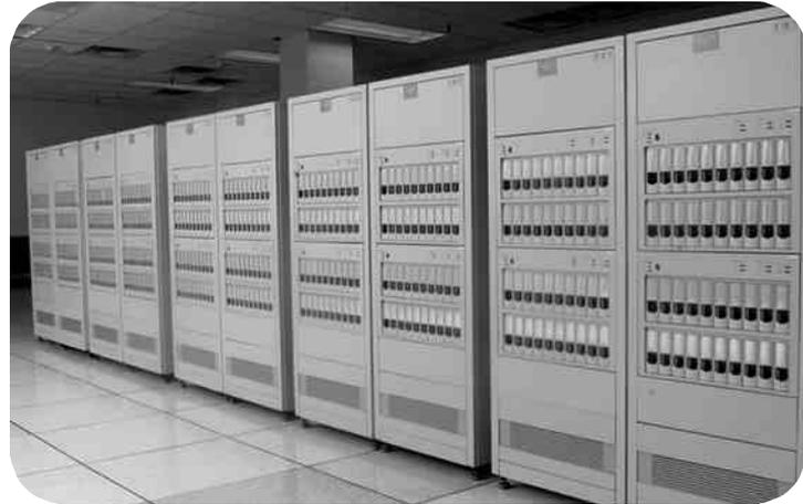
The Indiana Center for Database Systems (ICDS) received a donation from NCR and Wal-Mart of a Teradata database engine. The Teradata system has 80 processors, 20 gigabytes of memory, and 400 disk drives with an aggregate disk space of 1.6 terabytes.
